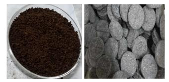
The calorific value of the pills and granules were calculated using the bomb calorimeter. Both the pellets have a calorific value of 12.3 MJ / Kg. This fuel pellet has a calorific value comparable to the biomass energy obtained from groundnut (12.60 MJ/Kg) [13], cowpea (14.37 MJ/Kg) and soybeans (12.94 MJ/Kg) [14]. The combustion qualities of the fuel produced in this study is sufficient enough to produce the required heat for domestic cooking and also for industrial
