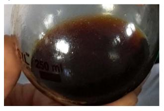
The solvent recovery was high (89%) and with proper measures can be as high as 99.9%. The extraction time was lower when muslin cloth with used compared to starch paper. The oil yield was higher in the case of muslin cloth.
